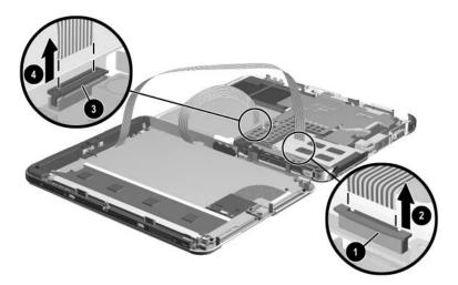
Disconnecting the Audio and Inverter Cables
